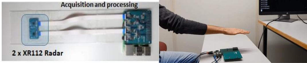
Fig. 1. The complete system used for recording and evaluation.
